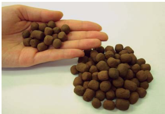
石炭灰人工骨材「Jライト」 Artificial Aggregate Made from Coal Ash (J-Lite)
