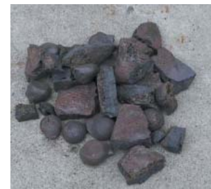
溶融結晶化骨材 Crystallized Aggregates
